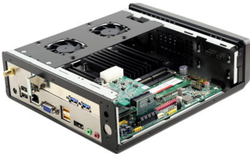
This set enables you to use a PCIe card (max. 16.5cm) in the M350 enclosure, when using together with Intel DN2800MT or Mitac PD10BI/PD10RI Half-Height ITX mainboard.
